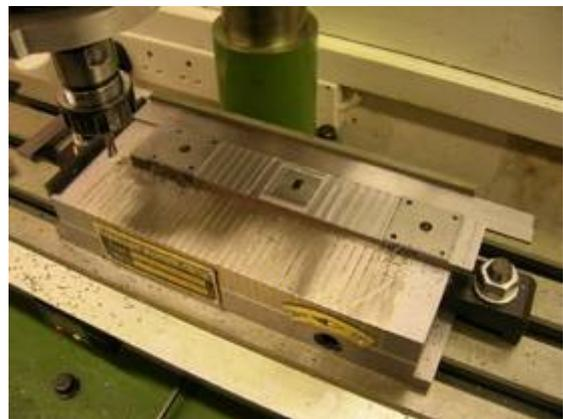
The final stage was to manufacture the buffers, the housing's of which had a square mounting base. I started off by taking 1.25" square bar, and boring a hole most of the way through it using a range of increasingly larger sized slot and end mills, finishing up with a boring head for the last 75thou on the diameter.
