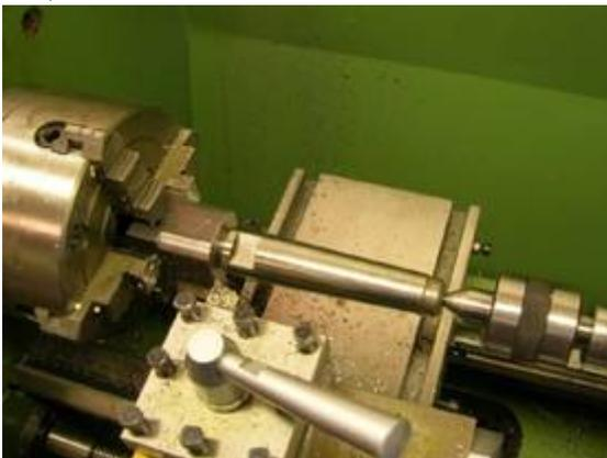
After finishing both buffer housings I swapped the chucks over and proceeded to turn the ends of the buffers from a 1.5" round bar and a 3/4" round bar, which I used as the arm protruding from the buffer housing. Once the buffers were completed I assembled my "kit" of parts to produce the completed tender chassis.
