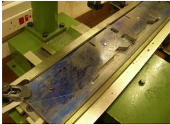
Unfortunately, my first learning experience was that by only machining one edge, both chassis frames warped and twisted, so my first effort was consigned to the scrap bin. This problem is partly due to the stresses induced during manufacture.
