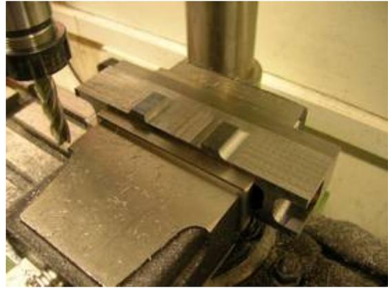
This buffer beam block was a particular challenge, as I used a fly cutter for the first time to reduce the thickness of the block down to 1.5" x 1.25". After this I proceeded to hollow out the block using slot and round nose mills.
