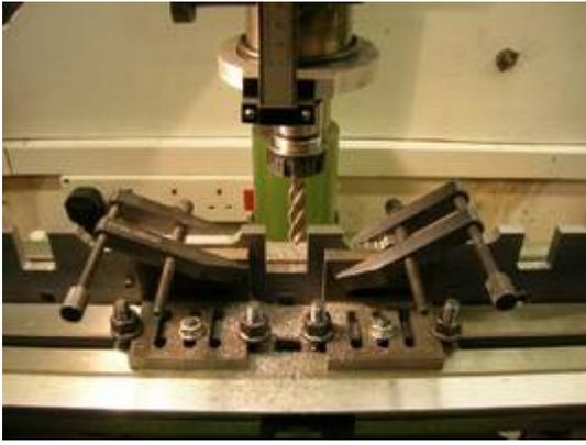
Next I machined all the frame stretchers. These all had to be milled to the same length, which I was able to do after some careful arrangement in the vice. As I was trying to build a semi-scale Q1, the outlines of the stretchers were along similar lines to those found on the real thing.
