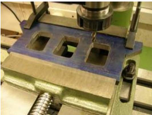
The most complex item was the buffer beam block, which I decided to machine from a solid 1.5" square bar, most of which was hollowed out. I believed that this block needed to be solid as, it supported the actual buffer beam, on which the sprung buffers and coupling hook were mounted, and a functional mount to hold the draw bar.
