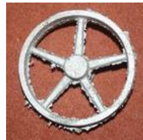
Figure 2, Zinc flywheel rough casting
