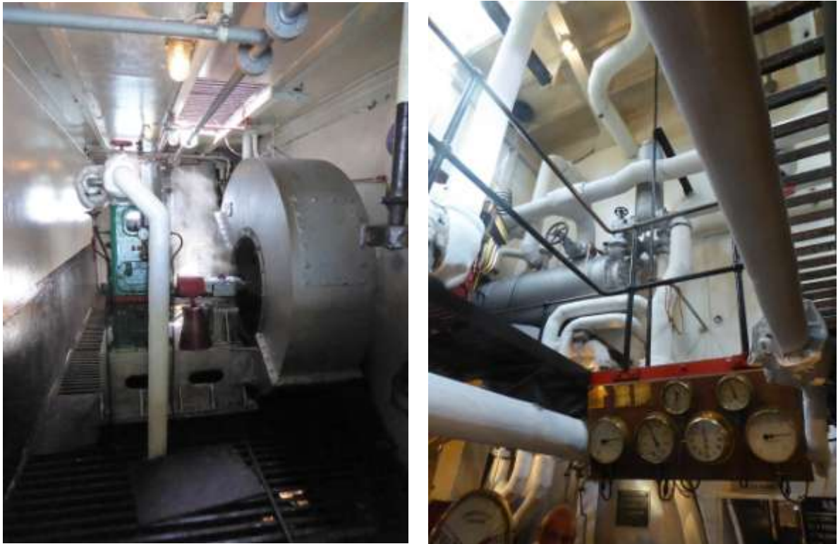
Above – the boiler room fresh air fan driven by a small steam engine and steam pipes from the boiler room
